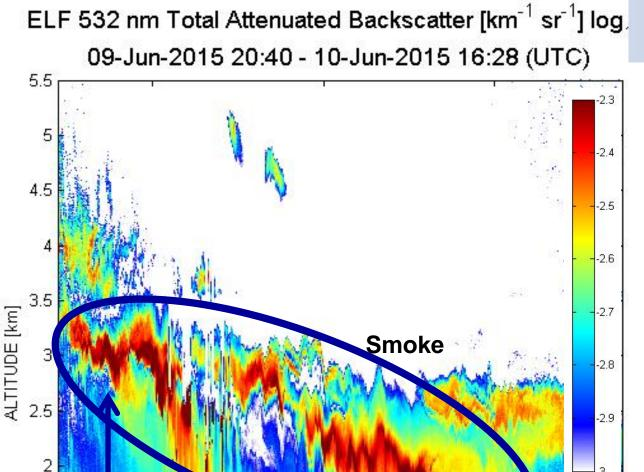
1.5 Smoke descended 3000m to reach Smoke at the surfac the surface 0.5 00:00 06:00 12:00 TIME [UTC] LIDAR images courtesy Dr. Ruben Delgado, UMBC
