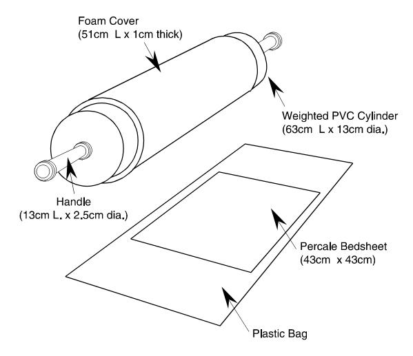
Figure B6-2. California Cloth Roller Sampling Device
