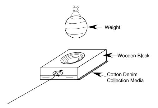
Figure B6-3. Dow Drag Sled Sampling Device
