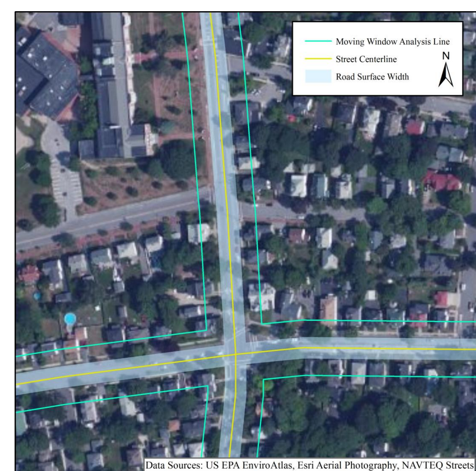
Figure 2. Road Buffers: To create the moving window analysis line, the road centerline (yellow) was buffered by the road width to create the road surface (transparent blue). The road surface was then buffered to create the analysis line (aqua).
