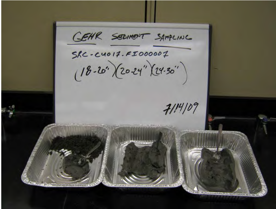
Representative Core from First Inventory Pass: SRC-FI-000007(18-30 inches)
