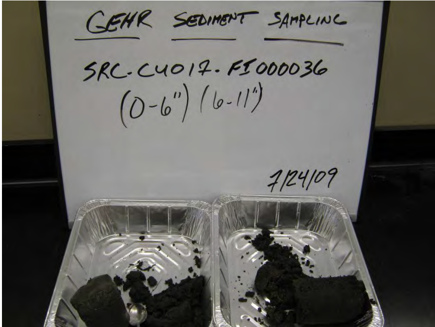
Representative Core from First Inventory Pass: SRC-FI-000036(0-11 inches)
