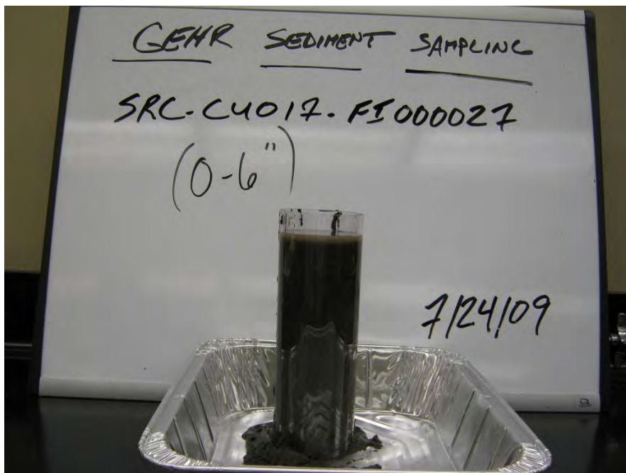
Representative Photo Showing Disturbed Residual in Core: SRC-FI-000027
