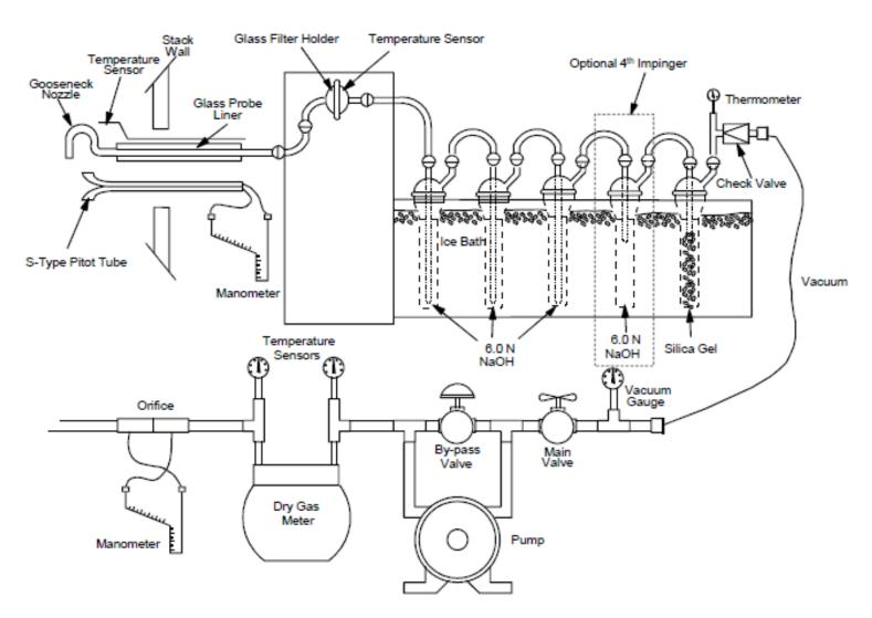
Figure 1. HCN Sampling Train, NaOH Configuration
