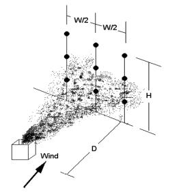
Figure 2. Illustration of Fixed Point Source Sampling Array
