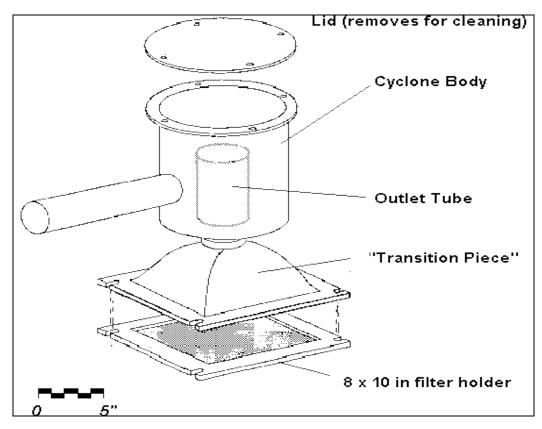
Figure 3. High-Volume Sampler with Cyclone Preseparator
