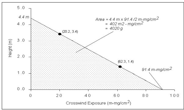
Figure 7. Vertical Integration of the Crosswind Exposure Values
