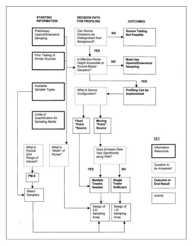
Figure 1. Decision Process for Profiling Applicability and Design
