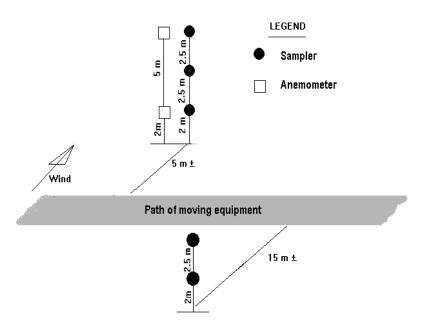
Figure 5. Example Sampling Array for Moving Point Source
