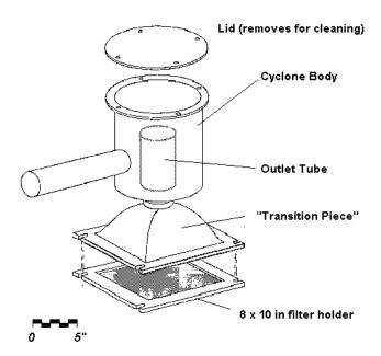
Figure 9. High-Volume Air Sampler with Cyclone Pre-Separator for Traditional Sampling of PM-10 from Dust Sources
