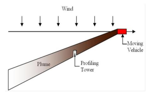
Figure 6. Illustration of Crosswind Plume Dynamics and Profiling Tower Location for Quantifying Emissions from Moving Point Source(s)
