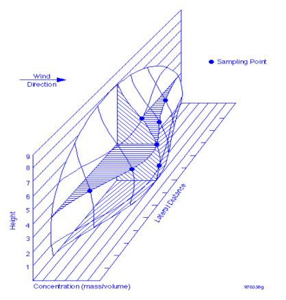
Figure 3. Illustration of Plume Concentration Profiles Downwind of a Fixed Point Source
