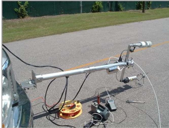
Figure A3-2. Mast in lowered position for assembly of components
