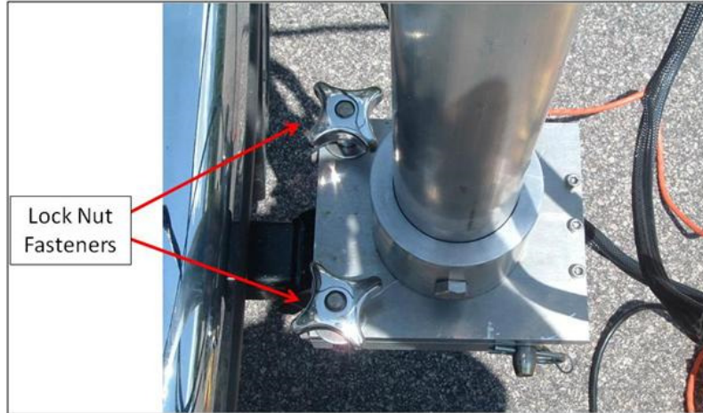
Figure A3-3. View of locked mast base plate
