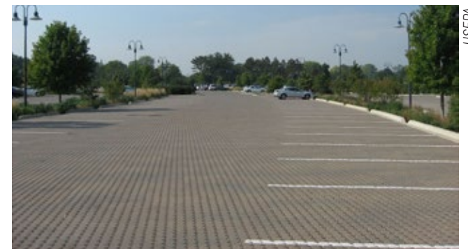
Permeable interlocking concrete pavement, Chicago, IL.
