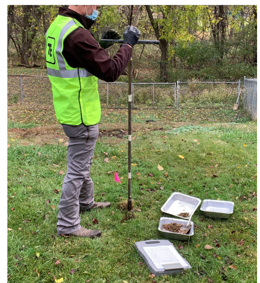
The photo below shows EPA's contractor taking surface soil samples from residential areas in Norwood in November 2020.
