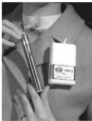
Radiation dosimeters of 1950s – “pocket screamer” and “chirper” from Oak Ridge National Lab
