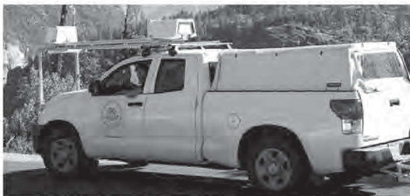
Figure A1.15 The MW-DOAS system mounted on the roof of a van, yielding sub ppb sensitivity for benzene and other aromatics.
