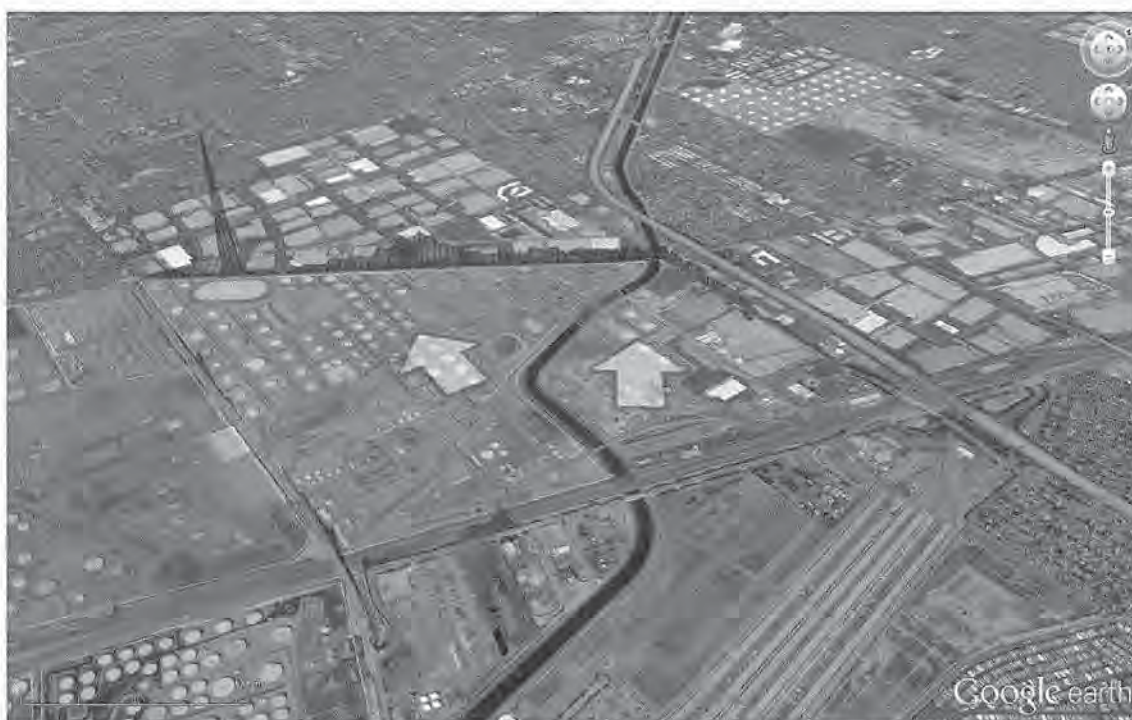
Figure 12 SOF 'box' measurement of the Tesoro Carson refinery on October 8 at 11:55 am. The shaded area in brown delineates the refinery area while measurements encompass a slightly larger area. Alkane column is shown as a blue curve with the apparent height being proportional to the gas column (5 m equivalent to 1 \text{mg}/\text{m}^2 , max 160 \text{mg}/\text{m}^2 ). Wind directions during the measurement are indicated by white arrows. North is to the upper right of the figure.
