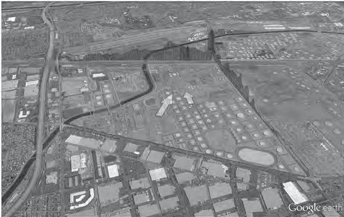
Figure 13 SOF box measurement of the Tesoro Carson refinery on October 7, at 13:55. Alkane column is shown as a blue curve with the apparent height being proportional to the gas column (5 m equivalent to 1 mg/m 2 , max 81 mg/m 2 ). Wind directions during the measurement are indicated by white arrows. North is to the lower left of the figure.
