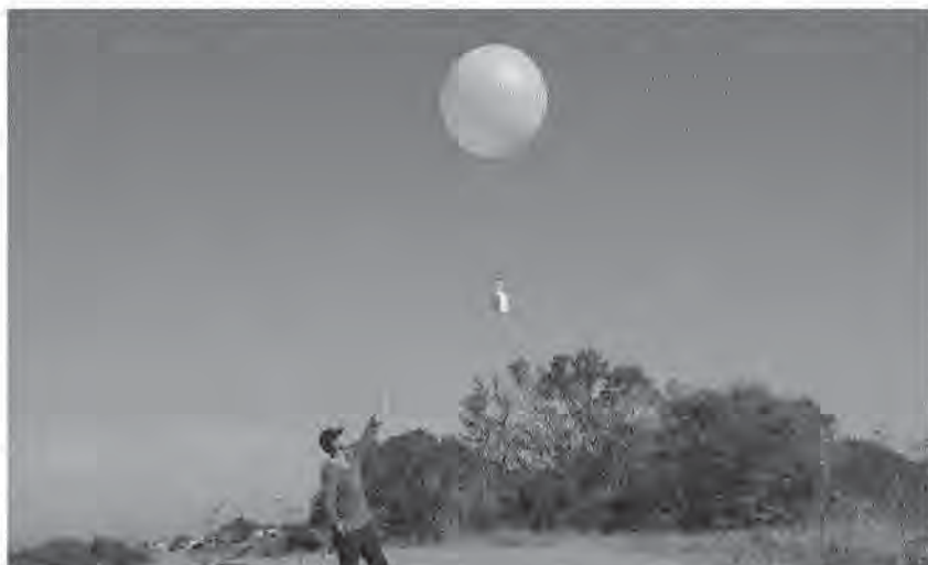
Figure 7 Sounding of the wind height profile by launching a weather balloon (I-met) during the campaign. The balloon drifts with the wind and sends its position measured with a GPS to a receiver.
