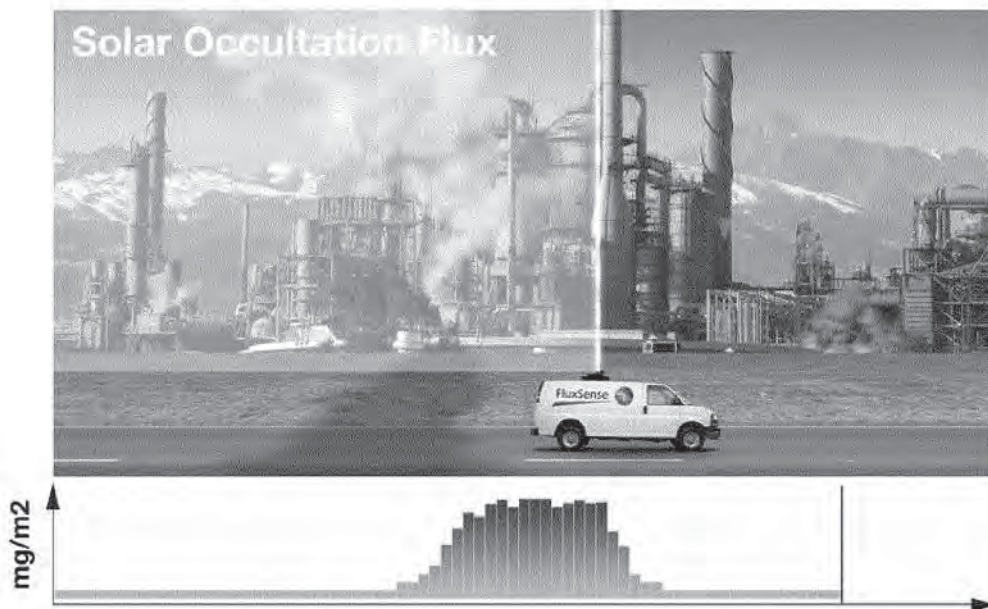
Figure 3 In the Solar Occultation Flux method (SOF) gases are measured by observing solar light in the infrared portion of the solar spectrum. The instrument is placed in a vehicle which is moved across the plume. From the accumulated mass measured across the plume the flux of gas is obtained by multiplication with the wind speed, see http://www.youtube.com/watch?v=6cre9q8YAzE
