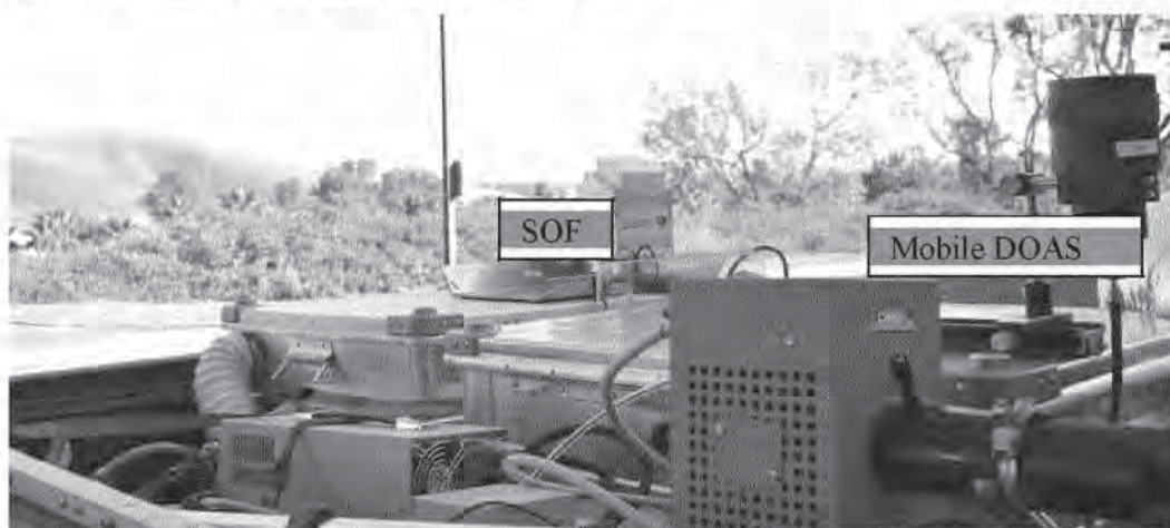
Figure 2 The SOF and the mobile DOAS systems. The solar tracker (front left) transmits solar light into the infrared spectrometer (mid right with a GPS on top) independent of the vehicle's position.
