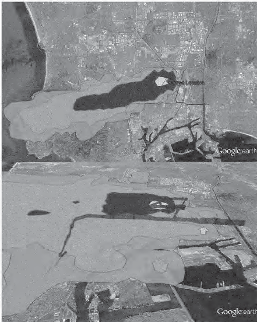
Figure 10 HYSPLIT dispersion model results (contours) for source located in Carson between 10:30 am and 13:30, on October 16, 2013. Also shown are SOF alkane measurements (blue curves). North is towards the top of the figure.
