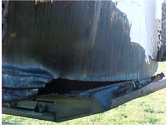
Fig 2 – Tank rupture detail.
