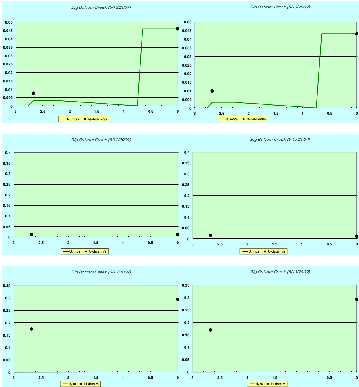
Figure B-11. Validations of observed and simulated flow (Q), velocity (U) and depth (H) in Big Bottom Creek
