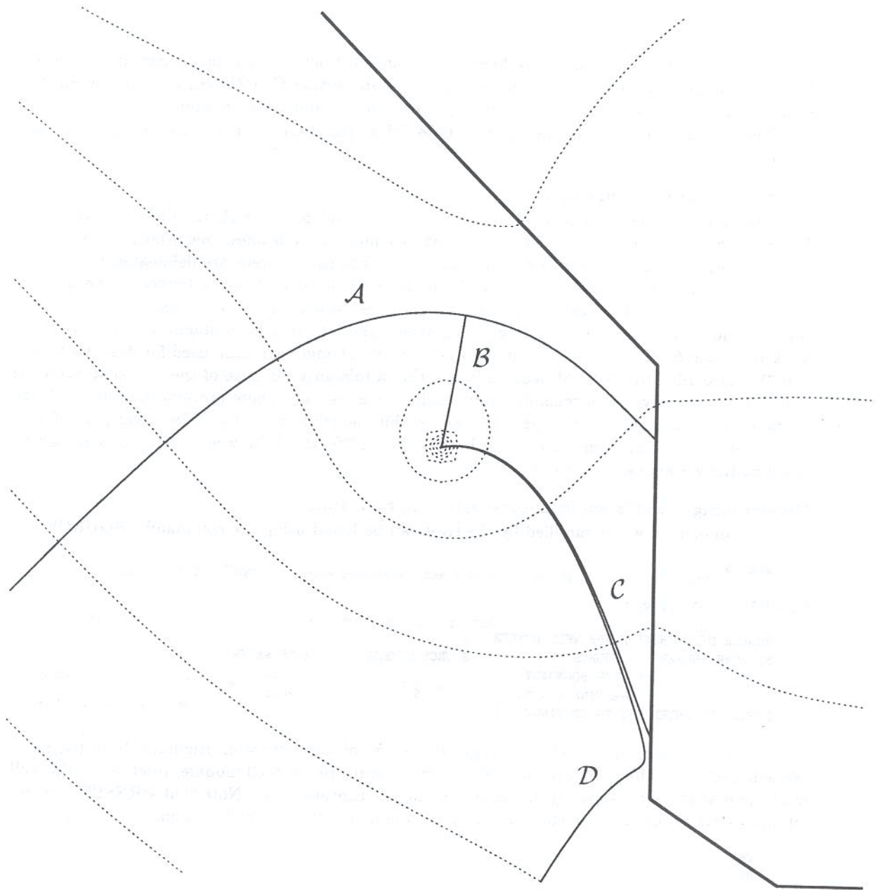
Figure 3.1 Capture zones generated for a well discharge of 1500 m 3 /day.
