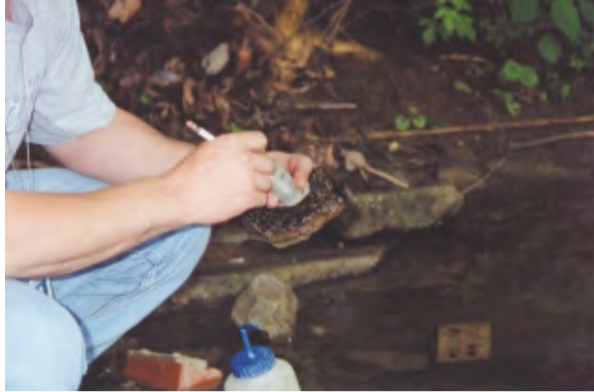
Figure 4-2. A member of a field crew dislodges attached periphyton from its substrate using the USGS-NAWQA method with the SG-92.
