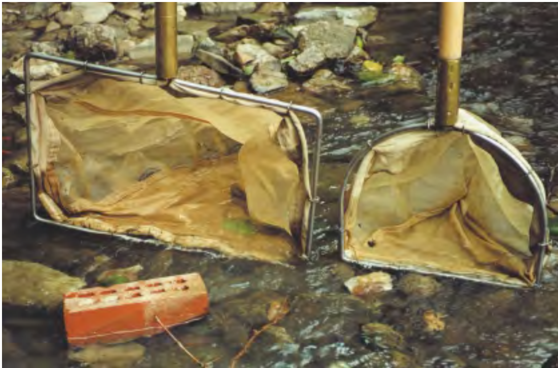
Figure 5-1. A modified kick net (left) such as is used in the USEPA-EMAP-SW protocols and a D-frame kick net (right) such as is used in the USGS-NAWQA protocols.
