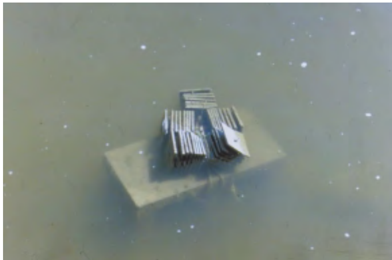
Figure 5-4. A Hester-Dendy sampling device placed in a river. Note: This sampler was set in a more shallow area for photographic purposes. Hester-Dendy samplers are normally set approximately 1 meter below the water's surface.
