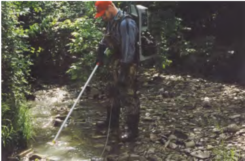
Figure 6-1. A field crew member uses a backpack electro-shocker to sample fish in a wadeable stream.
