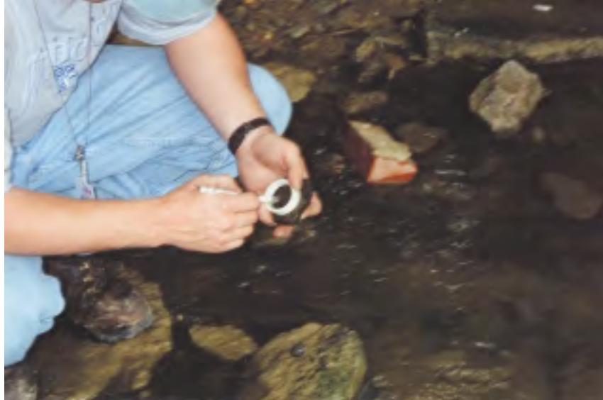
Figure 4-1. A member of a field crew dislodges attached periphyton using the EMAP-SW method.
