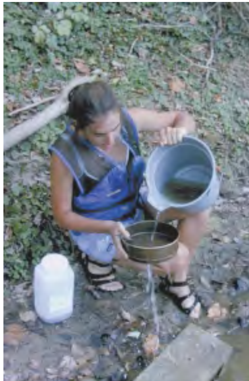
Figure 5-2. A fieldcrew member processes a benthic macroinvertebrate sample before it is transported to the laboratory for analysis.
