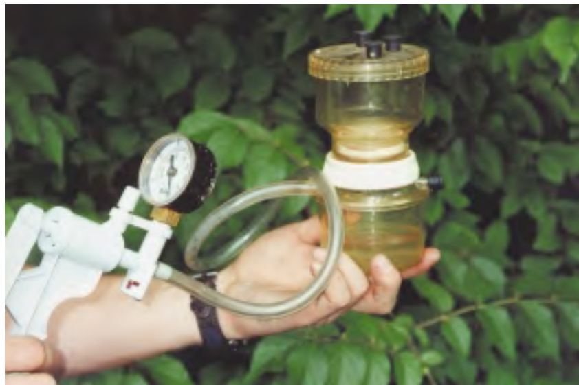
Figure 4-3. A field crew member filters a periphyton sample for chlorophyll analysis.
