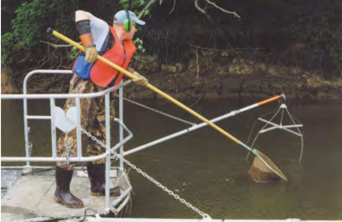
Figure 6-2. A member of a field crew samples fish using the boat-based electroshocking technique for boatable rivers.
