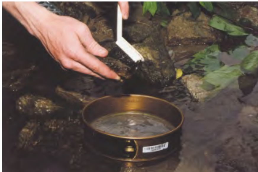
Figure 5-3. A field crew member uses a stiff-bristled brush to remove the attached benthic macroinvertebrates from a rock.
