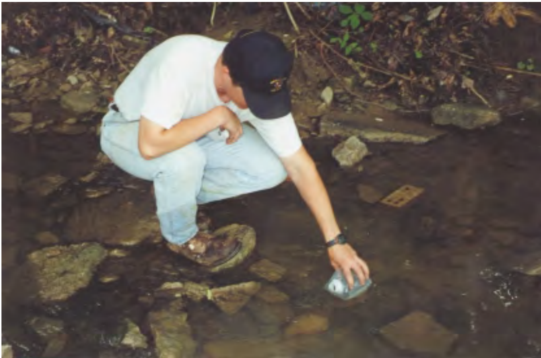
Figure 3-1. A member field crew member fills a cubitainer with water that will be used in water chemistry analysis.
