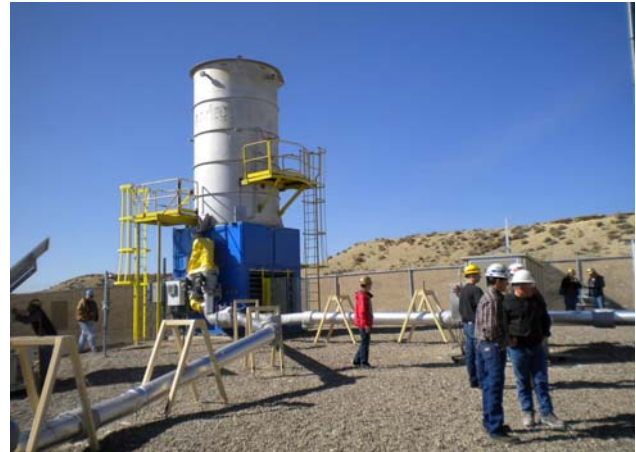
A close-up look of the CMM incinerator at the Solvay Mine site Photo: Mark Grady, ERG Courtesy of: Solvay Chemicals
