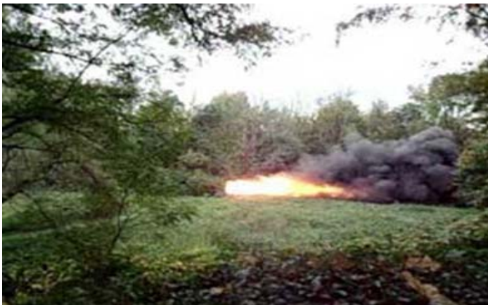
Controlled coal dust explosion on the grounds of the "Barbara" Experimental Mine Photo: GMI Newsletter
