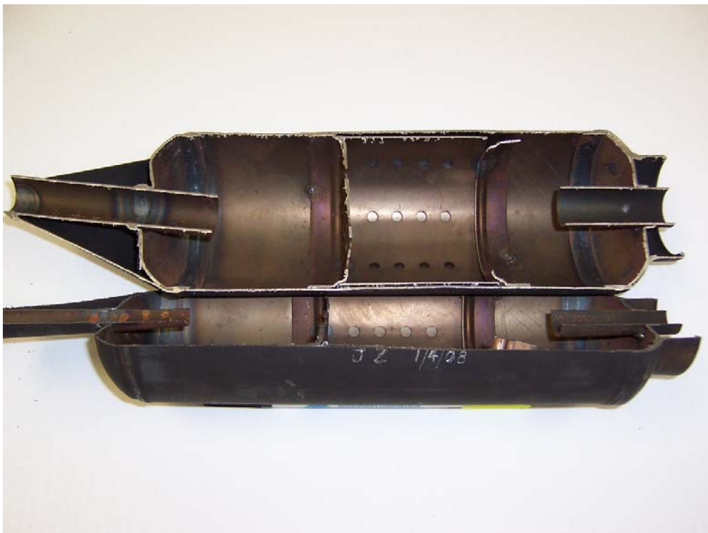
Muffler/ exhaust system missing catalyst
