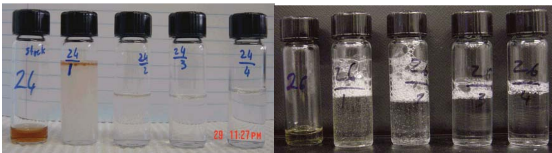
Figure 3. Precipitation of Test Chemicals when the Primary Stock is Diluted in TEGD Buffer. Compound 24 is 4-heptyl-phenol (CAS #1987504), and Compound 26 is dodecylbenzene sulfonic acid (CAS #27176870)
