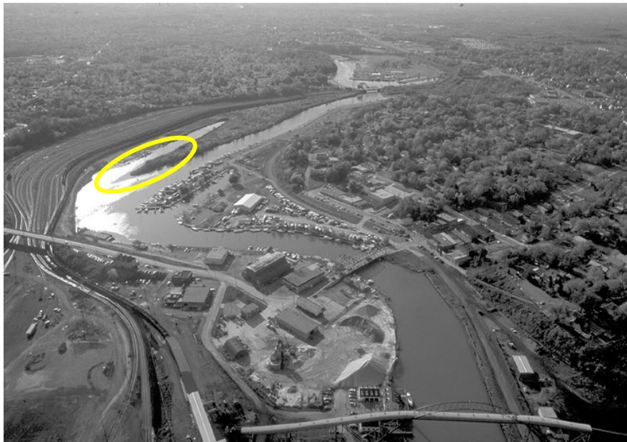
The 2005-2007 Legacy Act cleanup of the Ashtabula River removed 25,000 pounds of PCBs and other contaminants. Habitat mitigation is taking place near the 5 ½ slip, the area circled in this aerial photo.
