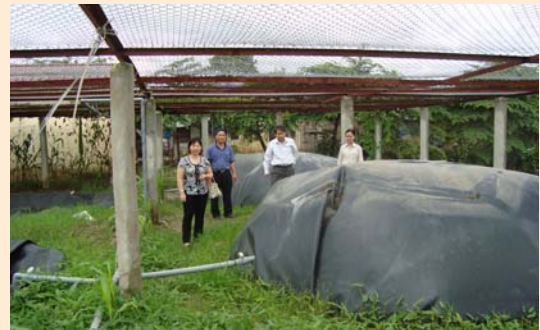
An anaerobic digester in northern Vietnam's Tu Duong village helps provide fuel for the kitchen.
