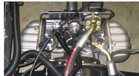
Primary rear drive in EPA's hydraulic hybrid UPS demonstration vehicle
