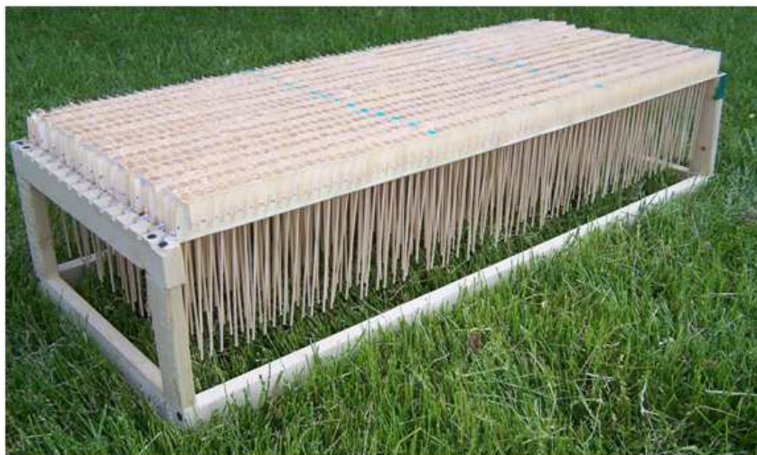
Figure 6. Carrier for 14 pre-labeled Al rods and pre-labeled linear cell array containing 1000 cotton swabs ready for field sampling
