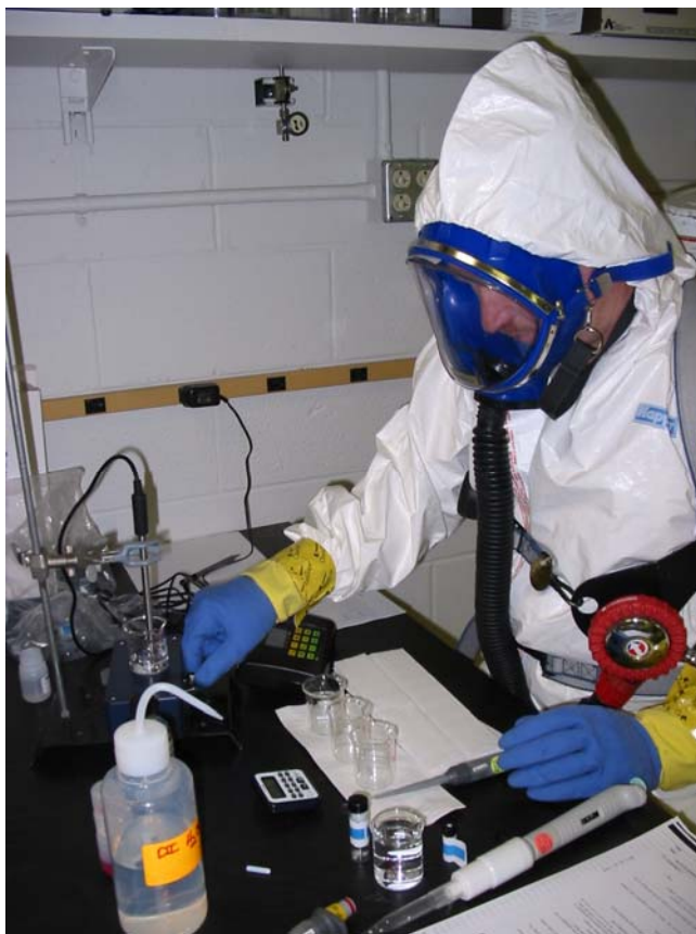
Figure 6-2. Testing of the Neuro-IQ Tox Test Kit™ with the Non-Technical Operator Wearing PPE
