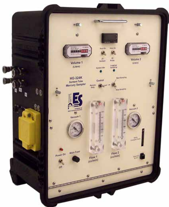
Figure 2-1. HG-324K Sorbent Tube Mercury Sampling System
