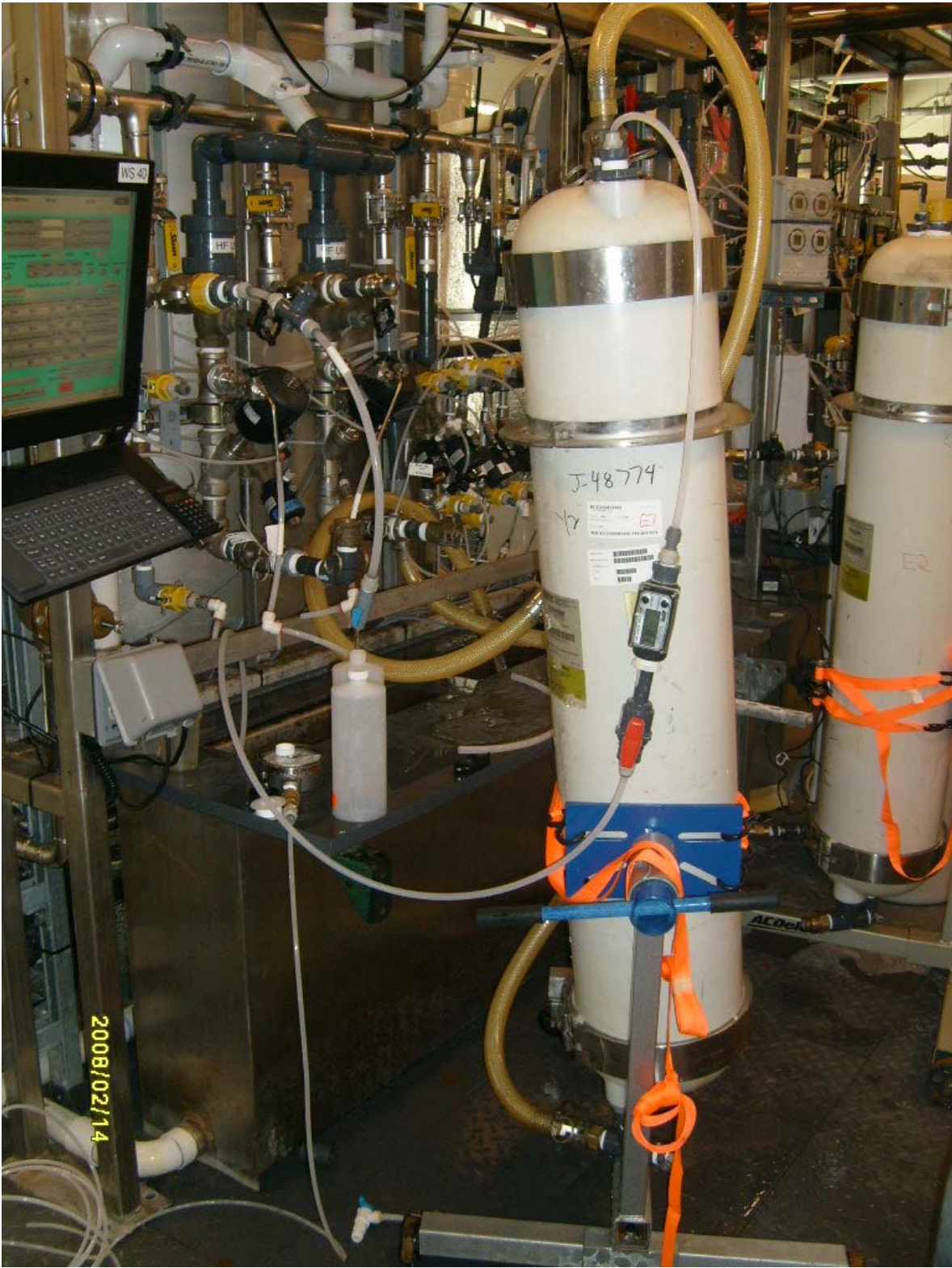
Figure 3-1. UF modules plumbed to test station in NSF testing laboratory.
