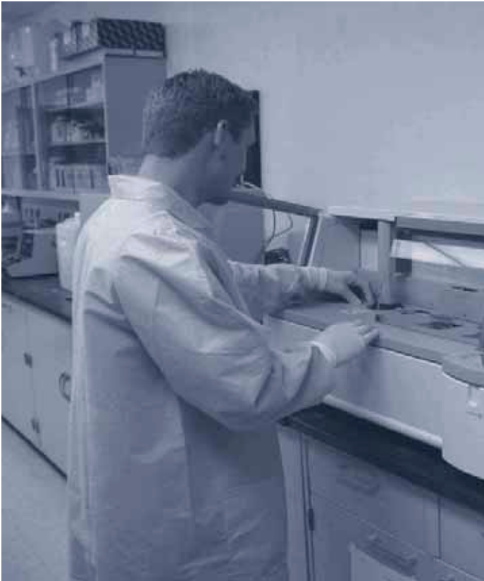
Here, a water quality analyzer is being used to determine the chemical composition of Rio Grande River water.
