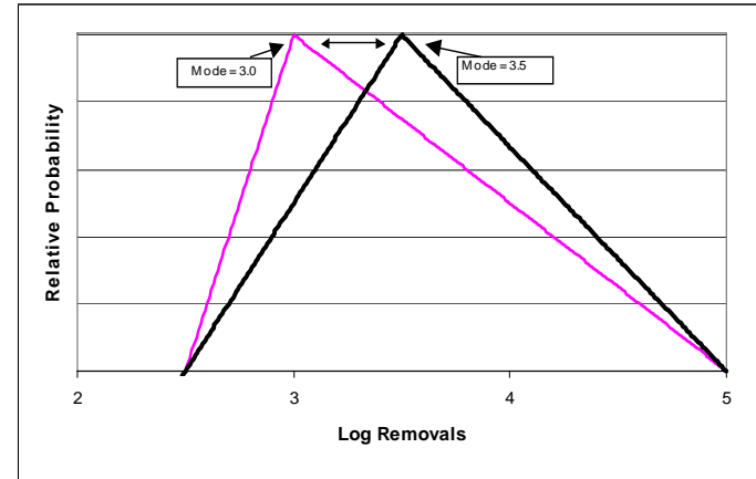
Exhibit 4.20d: Distribution of Cryptosporidium Reduction in Large Systems Pre-LT2ESWTR, Estimate With 0.5 Log Reduction Credit
