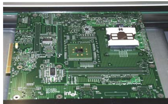
Figure 2. Reflow test PWB assembly
