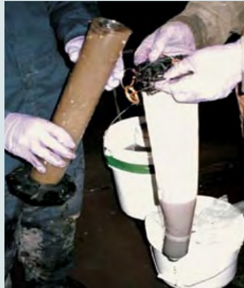
Ballast sampling includes collection of water and sediment samples to examine the diverse collection of phytoplankton and other invertebrate fauna (courtesy of NOAA Great Lakes NOBOB Assessment Program).
