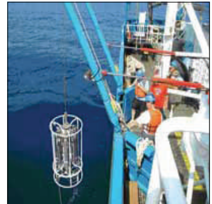
Coastal Science Team lowering a water quality sampler into the Atlantic Ocean
