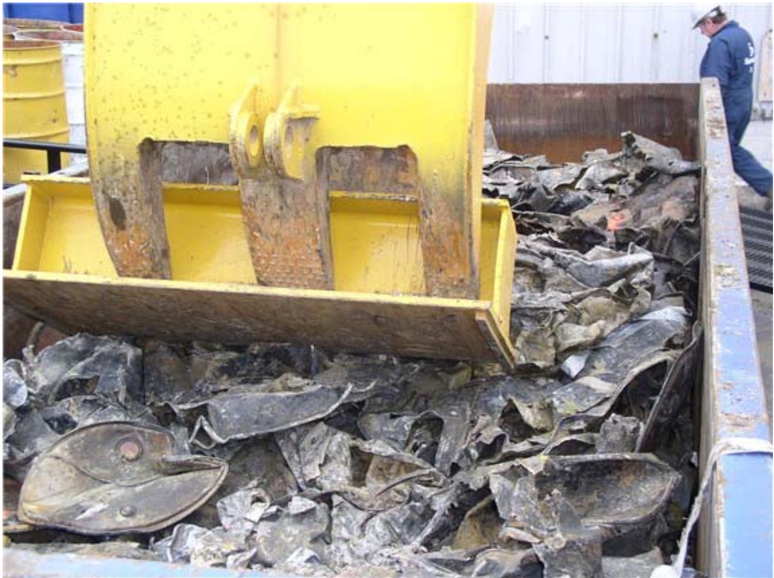
Empty drums are crushed and bulked together for shipment off Site.
