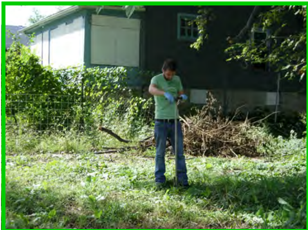
An EPA contractor uses a bucket auger to collect soil. The soil will later be sent to the EPA Region 7 lab where it will be analyzed for contaminants.
