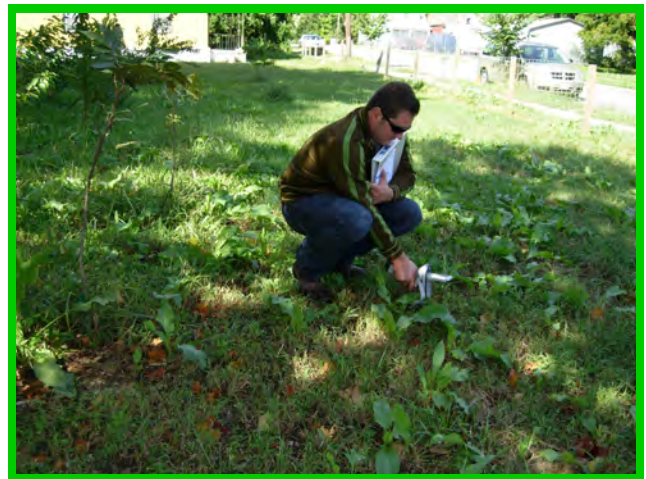
An EPA contractor uses a handheld XRF analyzer to examine the content of heavy metals within the soil at a future garden site in Kansas City, MO.
