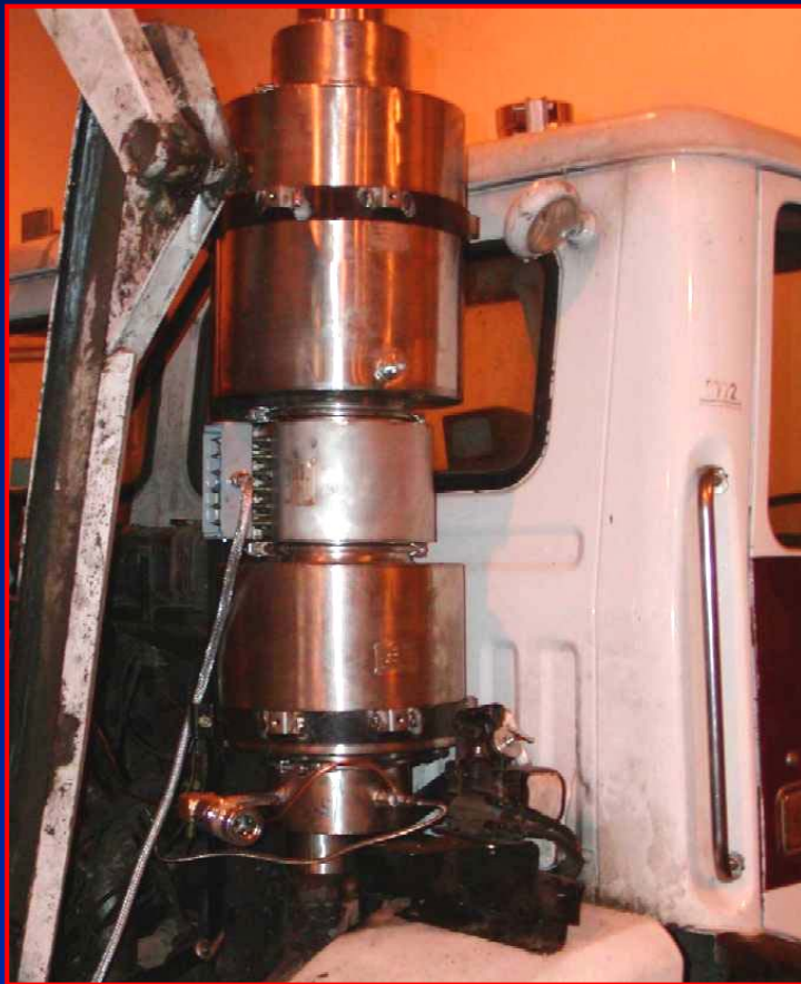
Catalyst-Based Filter with Electric Heater Assist
