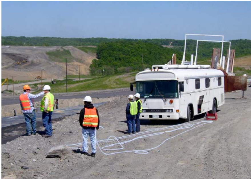
Chicago (May 28, 2008) - U.S. Environmental protection Agency's TAGA bus (Trace Atmospheric Gas Analyzer), a specialized mobile air quality laboratory, visits the Countwide Landfill in East Sparta, Ohio.
