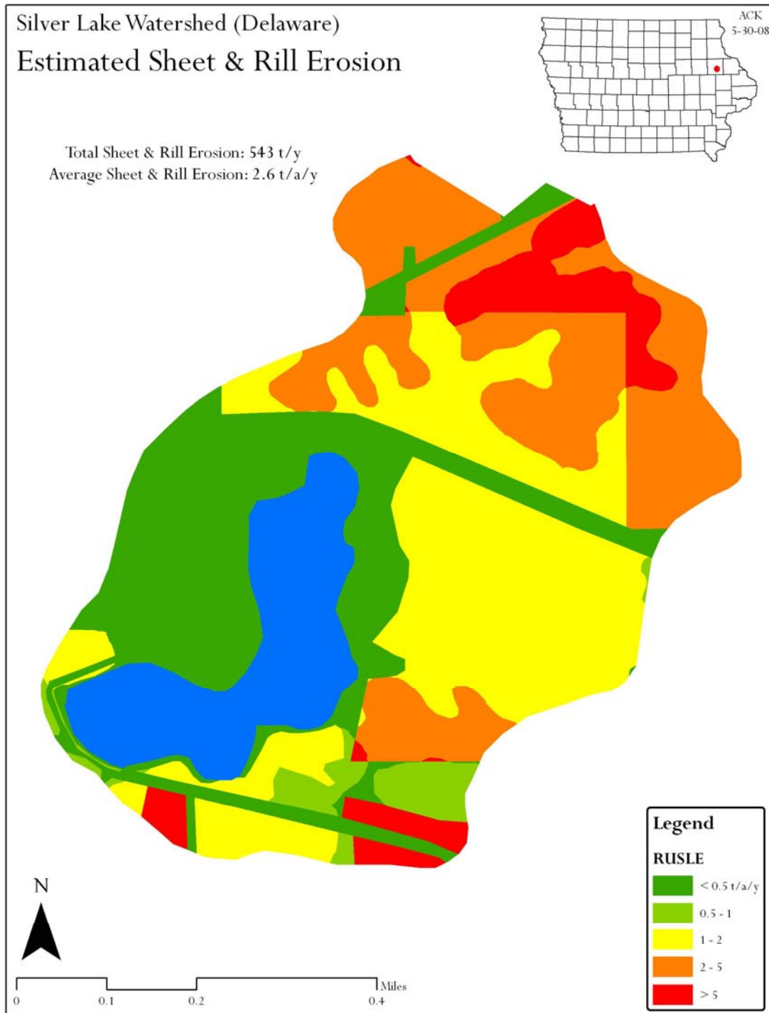
Figure E-1. Estimated erosion within Silver Lake watershed with current land use and conservation practices
