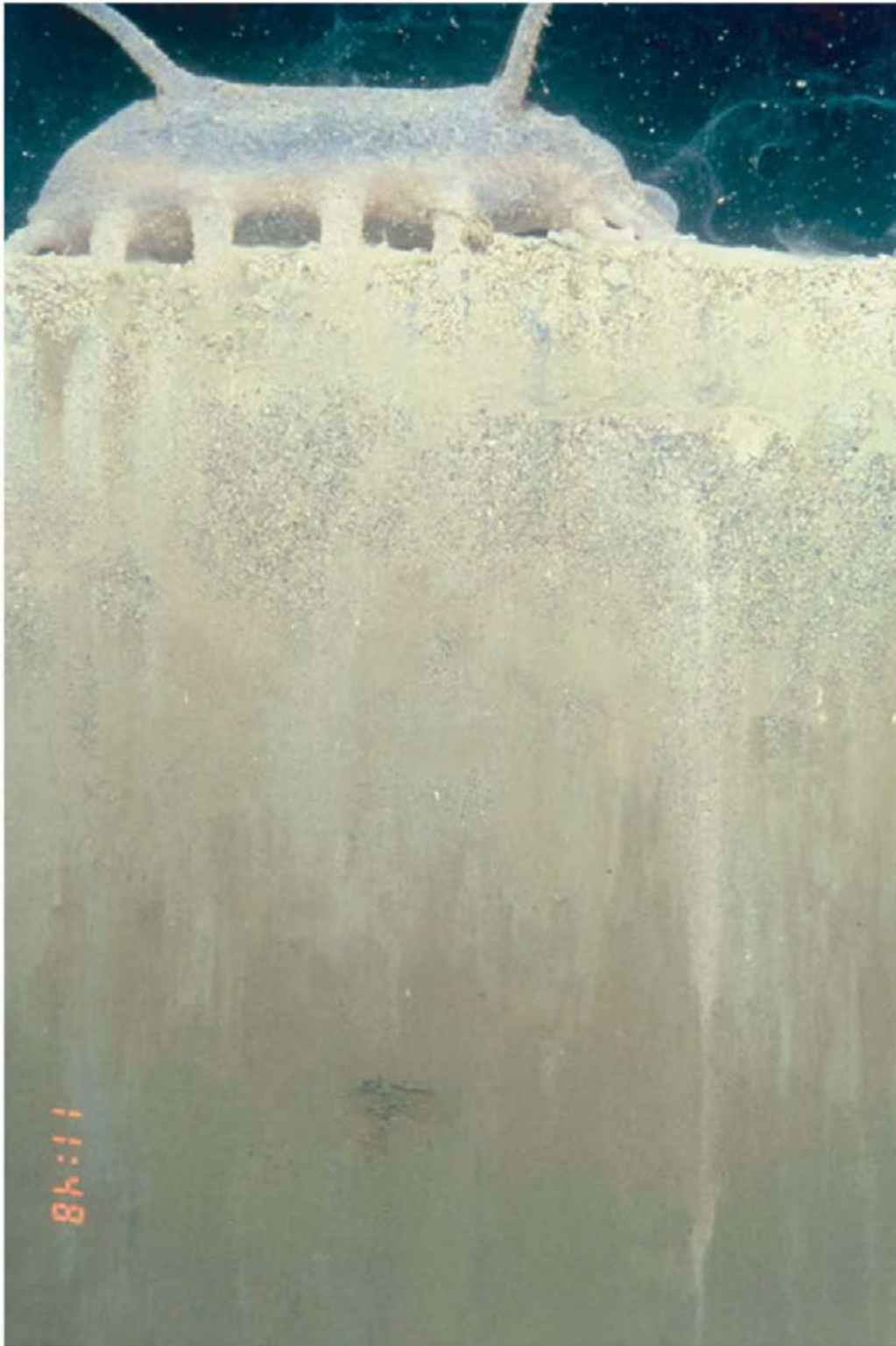
Figure 10: Sediment profile image from SFDODS taken within the boundary during the 1997 survey (Station 9) within the boundary shows evidence of a distinct layer of dredged material and an epibenthic animal grazing on the surface (elasapoid holothurian, Scotoplanes globosa ). Scale: width of profile image = 14.5 cm.
