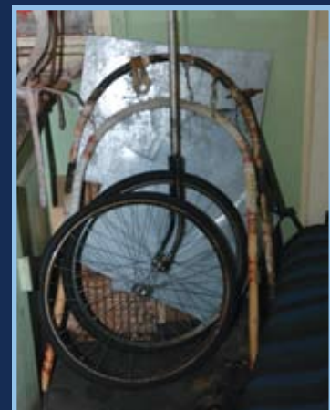
Bicycle wheels used to make sledge meters to measure the distance run
