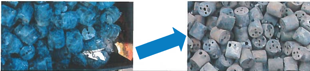
Hazardous materials were safely and successfully thermally treated to remove explosive and toxic hazards resulting in materials which were safe and clean.
