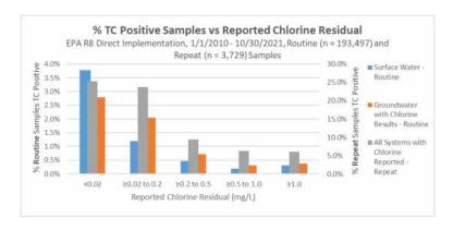
EPA Region 8 recommends that all systems, including groundwater systems, maintain a minimum chlorine residual of 0.2 mg/L free chlorine or 0.5 mg/L total chlorine throughout the distribution system. This recommendation is consistent with the results of the above analysis.
