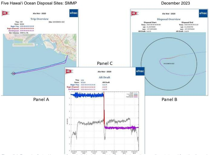
Figure 7-6. Example of a tracking report for an individual disposal trip. Panel A shows the vessel's route to and from the disposal site, with the blue line indicating the vessel is loaded and purple indicating it is empty following disposal. Panel B is a closeup of the disposal site's SDZ, showing the disposal (in red) occurring fully within the zone. Panel C shows the vessel's draft and speed throughout the trip, confirming no substantial loss of material from the vessel during transport.
