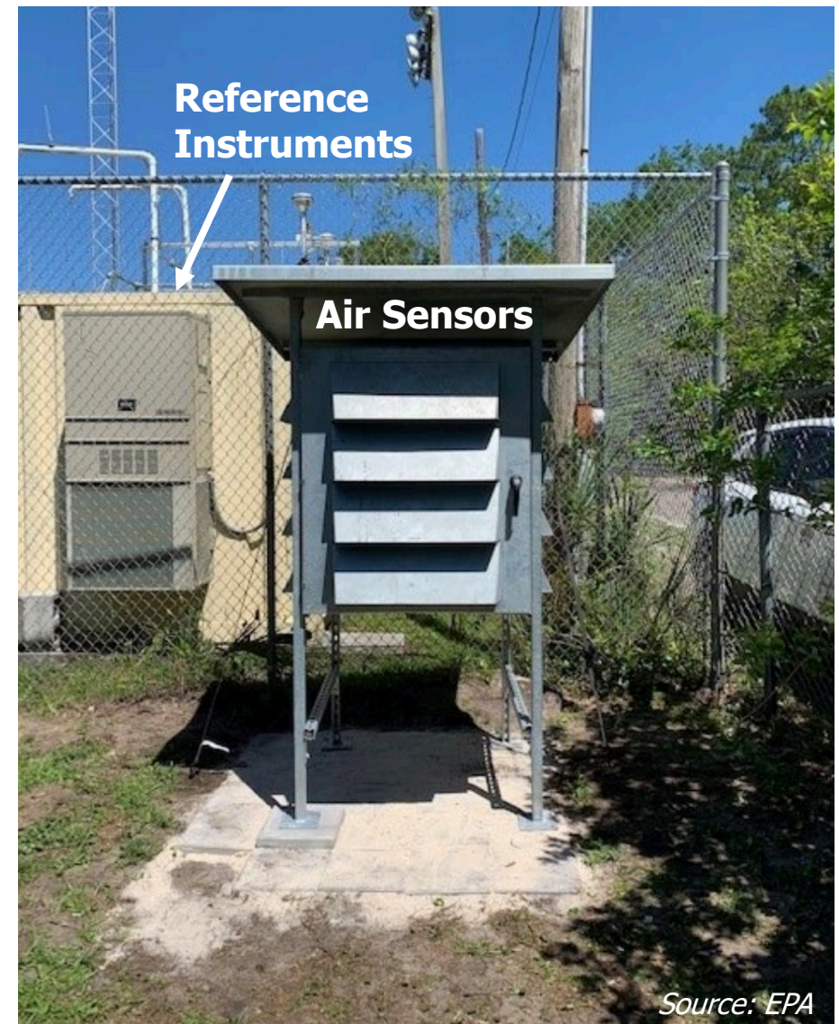
Collocation Shelter installed in Jacksonville, Florida
