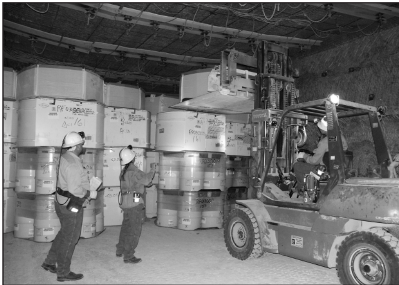
Magnesium Oxide being placed on top of a stack of contact-handled transuranic waste at WIPP.
