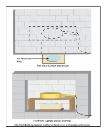
Suggested configuration for rapid screening of air particulate filters
