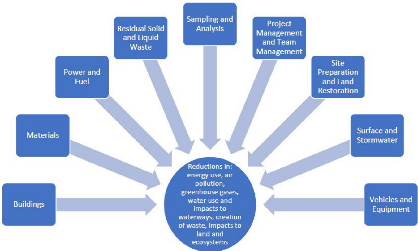
Figure 1 – Boxes represent each cleanup activity category in the ASTM Standard Guide. Implementation of BMPs from these categories directly affects the Core Elements of EPA's Principles for Greener Cleanups in the center circle.
