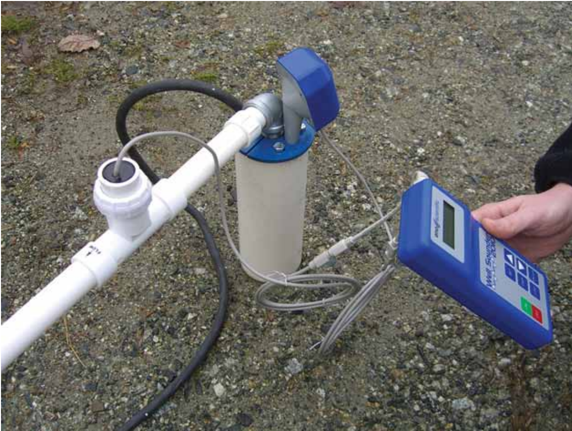
Figure 6: Portable Water Meter
