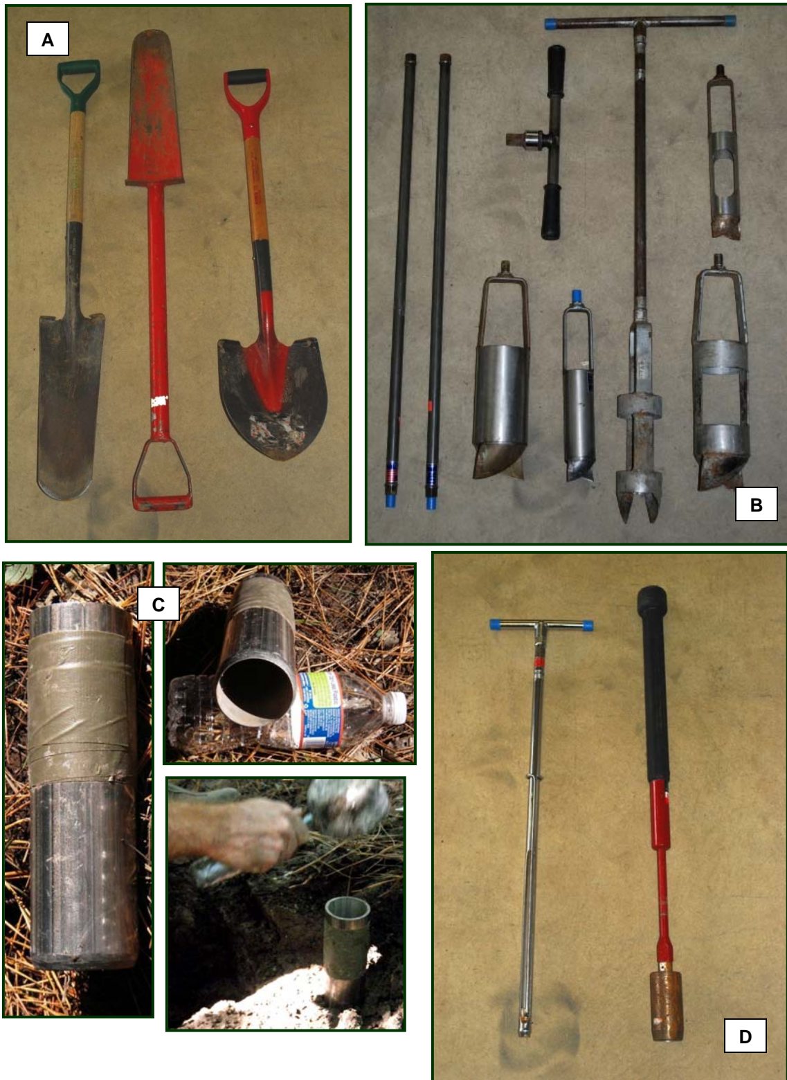
Figure 6-2. Examples of Tools for Soil Pit Excavation or Soil Extraction. Photos by Gregg Lomnicky. A. (Left to right) Tiling, Sharpshooter, Regular Shovels. B. (Left to Right) Auger handle extensions, ratchet handle, mud auger buckets (solid), bucket auger with handle, auger buckets. C. Bulk density corer (steel tubing with beveled edge). D. (Left to Right) Soil Probe, Hammer Corer. The tools most commonly used in the NWCA are a tiling or sharpshooter shovel (A) and an auger (B) for pit excavation and chemistry sampling, and a can (see Figures 6-8 and 6-9) for bulk density sample collection. Other tools pictured (C and D) may be useful for specific conditions and may be available from a local soil scientist (e.g., see Text Boxes 6-2 and 6-6).
