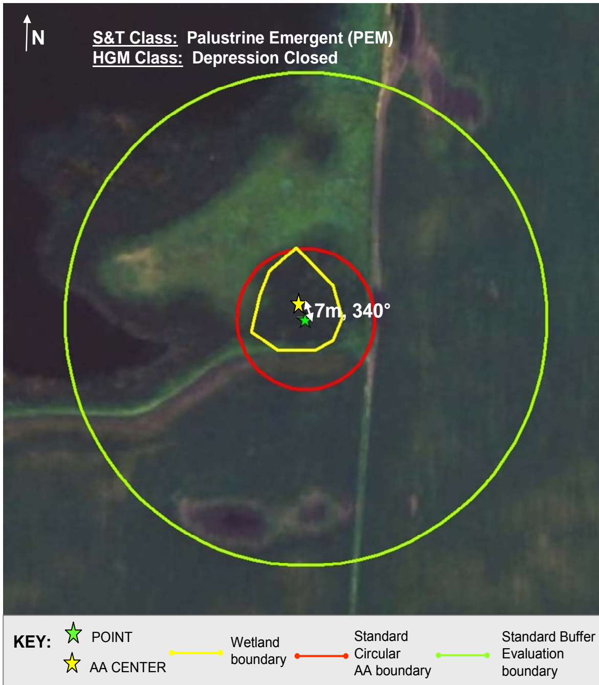
Figure 3-4. Example of a Wetland Boundary AA layout (see Section 3.2.2.2) depicted on an example aerial photo as would be found in the site packet. Distance and bearing from the POINT to the AA CENTER are indicated. The Standard Circular AA layout and the Standard Buffer Evaluation boundary are shown for comparison.
