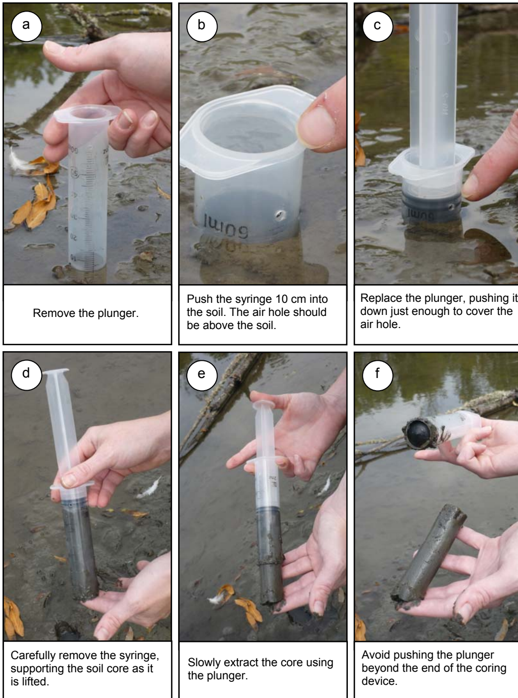
Figure 6-6. Extracting a soil core for an isotope soil sample or sediment enzyme sample. Photos by Casey Pollock and Amanda Nahlik, USEPA.
