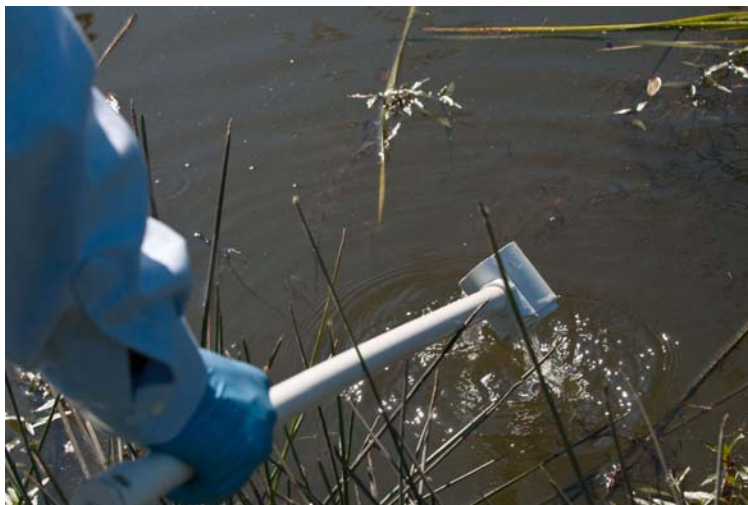
Figure 8-2. Example of long-handled dipper in use for sampling surface water. (Photo credit – U.S. Environmental Protection Agency, Eric Vance)
