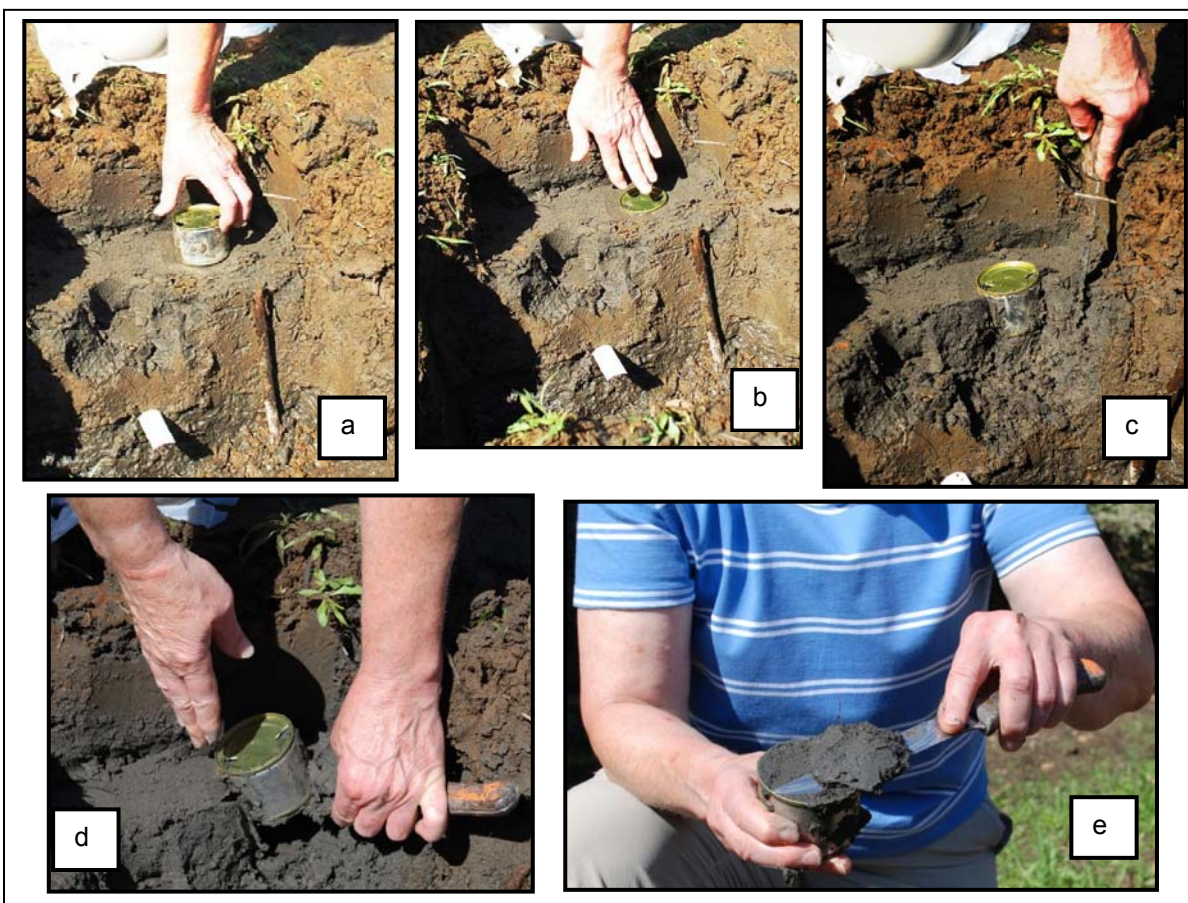
Figure 6-9. Collecting a bulk density core using a small can. Photos by Gregg Lomnicky.
