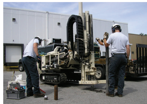
Conducting direct push soil sampling
