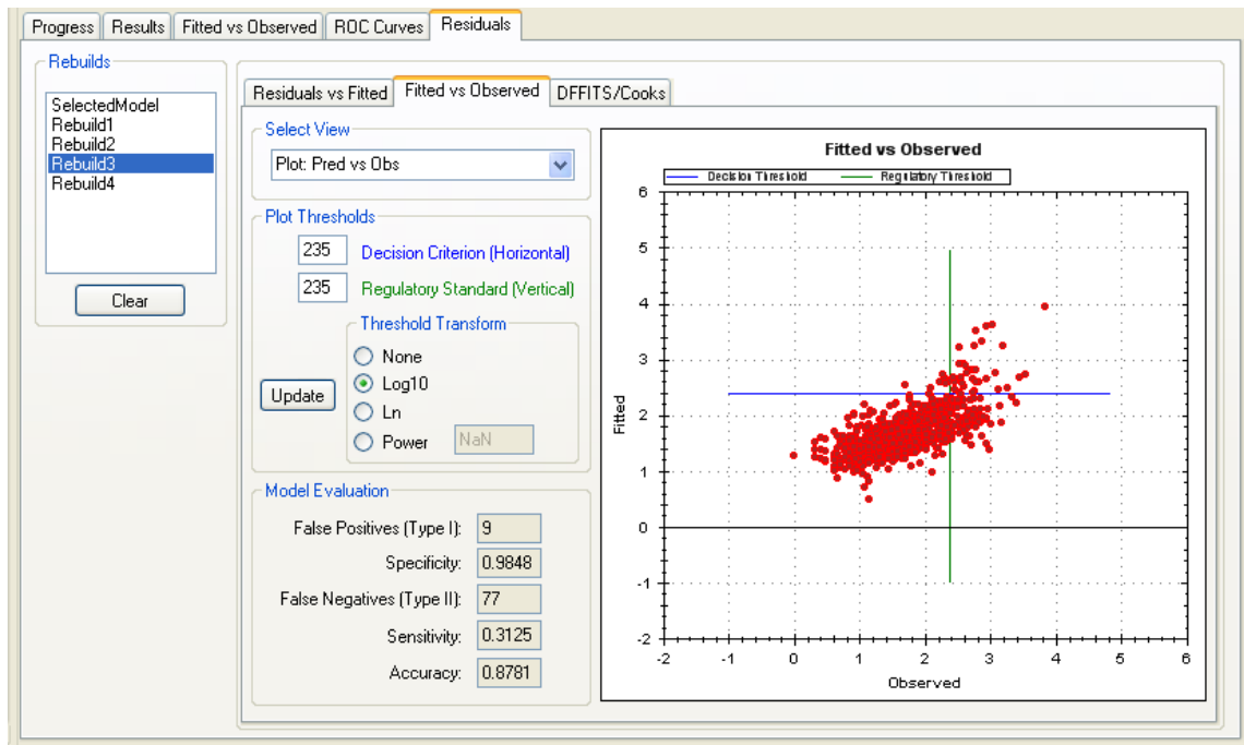
Figure 42. Fitted vs Observed plot on the Residual subtab with model evaluation threshold control and model evaluation statistics
