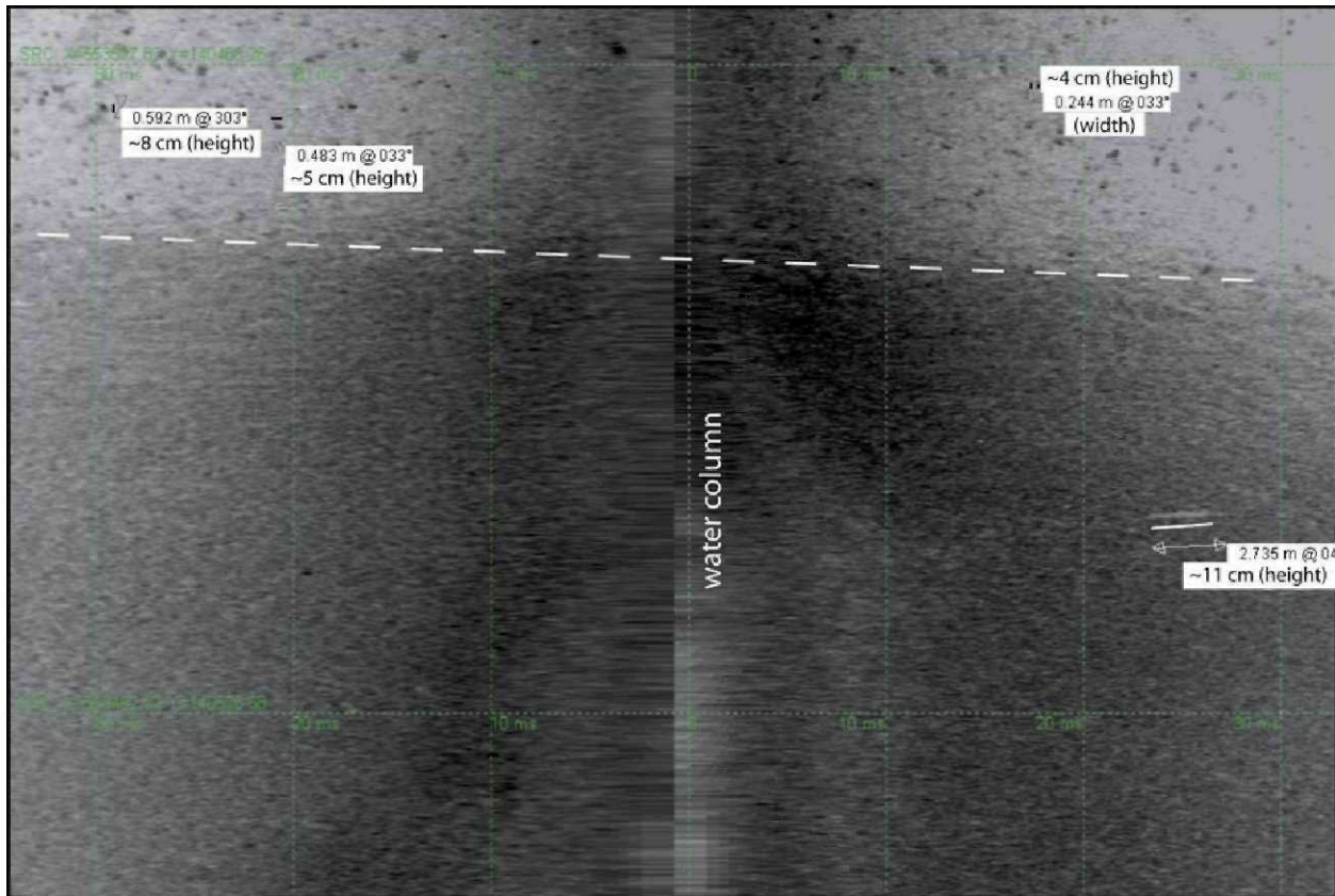
Figure 5: Example sidescan profile from the deeper portion of northwest quadrant. The transition from shallow to deep (lighter to darker) is noted by a dashed white line. Except where noted, all sizes in the figure refer to estimated lengths of individual features. Only a few example features are labeled because numerous features are present.
