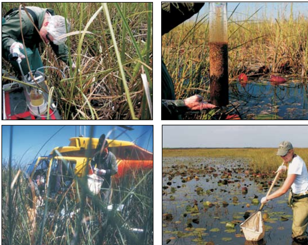
FIGURE 15. Biogeochemical sampling included surface water (top left), floc and soil (top right), and mosquitofish (bottom). The surface water sampling apparatus (top left) and soil coring device (top right) were designed and constructed for the Program.
