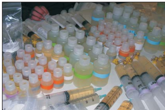
FIGURE 17. Surface water and pore water samples in the chain of custody lab at the end of a day's sampling. Samples were distributed to eight analytical laboratories for determination of mercury, nutrient, and ionic content.
